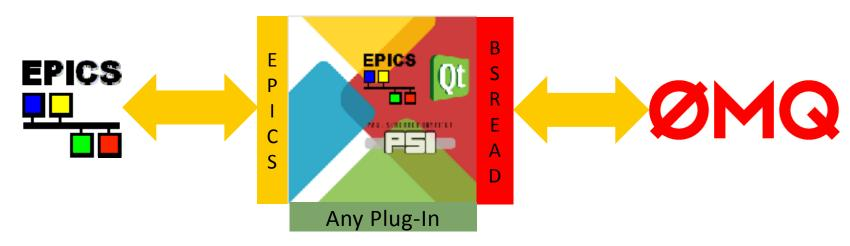
Actual plugins: EPICS 3.14, BSREAD (a beam synchronous data acquisition using Ø MQ), EPICS4 (obsolete old version, not really tested and not used), a demo plugin as simple example.
